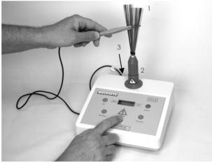
Fig.2 - Testing a diathermy instrument
